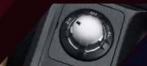
'Shift-on-the-fly' 4x4 Select Dial for Fingertip Terrain Control
