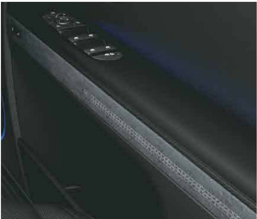
Look closely at the detailing on the door and you'll find 100% recyclable paperette. Made from HDPE, it has the same lightness and texture of traditional paper.
