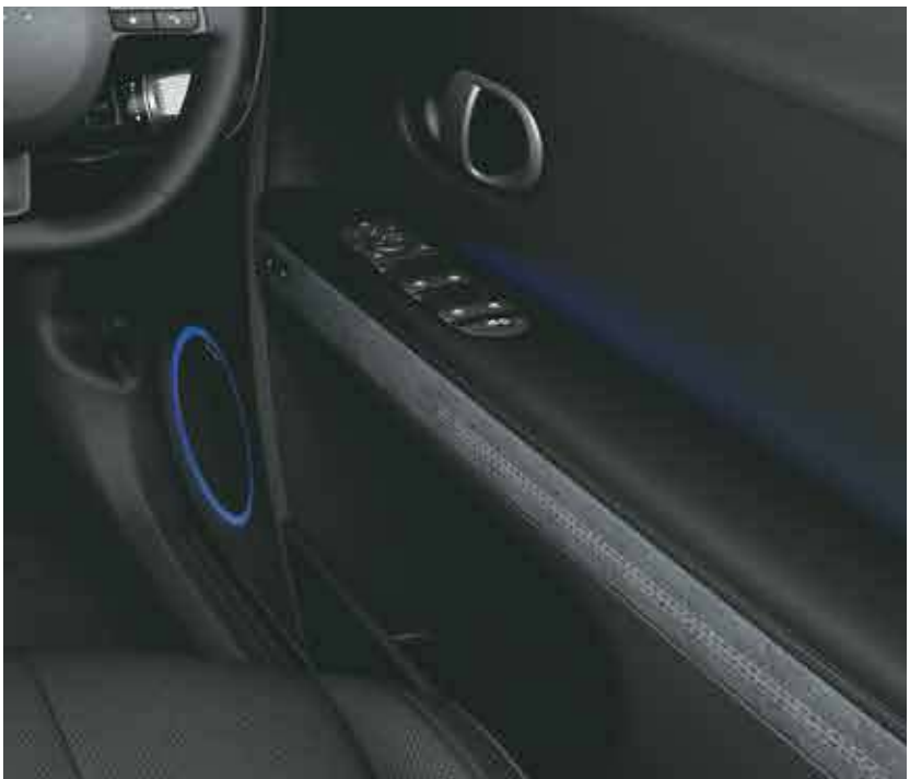
For each Hyundai IONIQ 5, recycled bottles are shredded into plastic chips that are used for seatback and door armrests.
