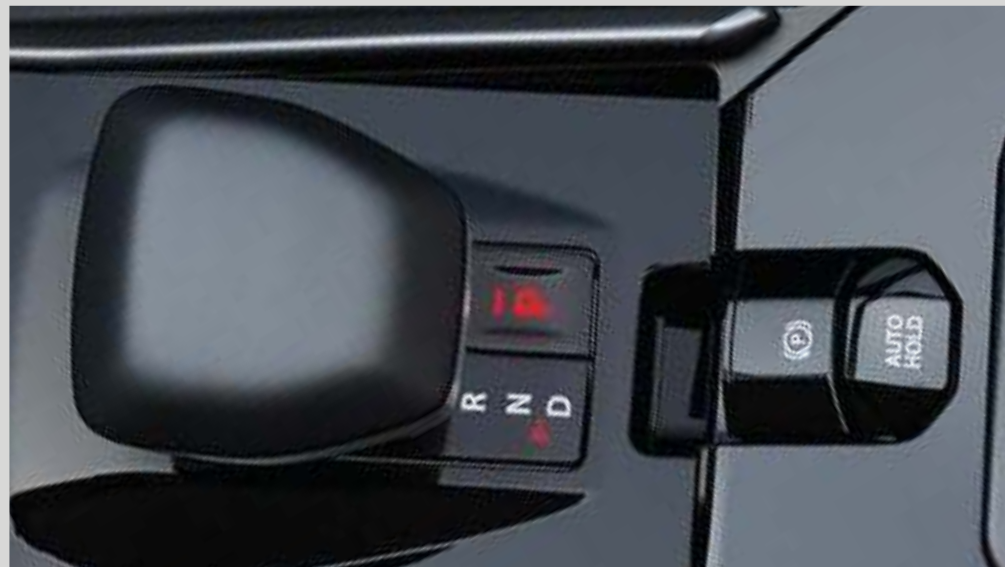
JLR DERIVED COMMAND SHIFTER (AT) ELECTRONIC PARKING BRAKE (EPB) WITH AUTO HOLD 6-SPEED AUTOMATIC TRANSMISSION
